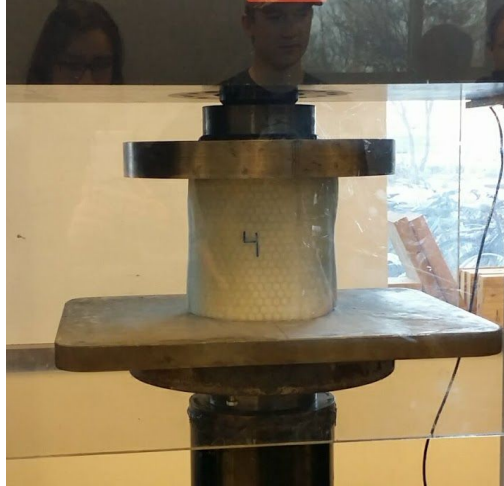
Figure 23. Compression testing of airframe cross-section.
