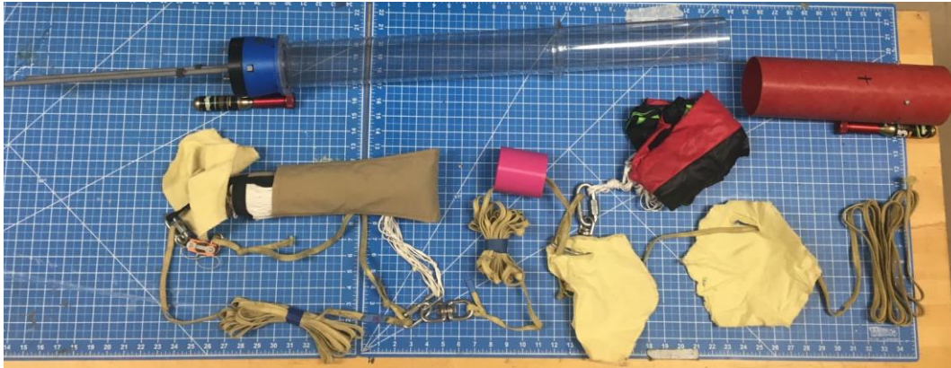
Figure 14. The disassembled recovery system ahead of a test launch.
