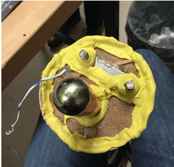
<CO2 system with tacky tape in test airframe, later tests>
