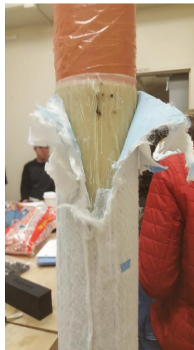
Figure 9. Bad quality surface finish of first layup
