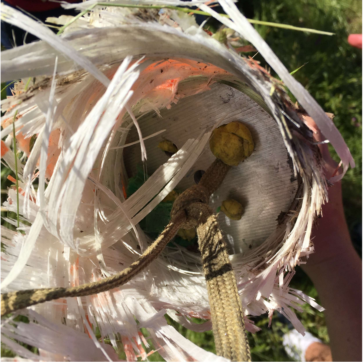
Intersection shock cord correctly attached to motor retainer, all holes plugged for pressurization
