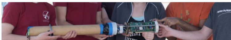
Figure 16. Integrated recovery + AV system shows that serial deployment allows for a more elegant system that is far more compact and simple without need for multiple breaks in airframe.
