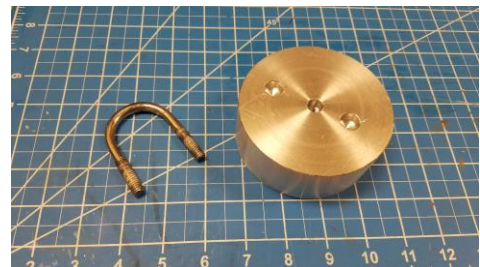
Figure 7. Aluminum Motor Retainer and U-bolt
