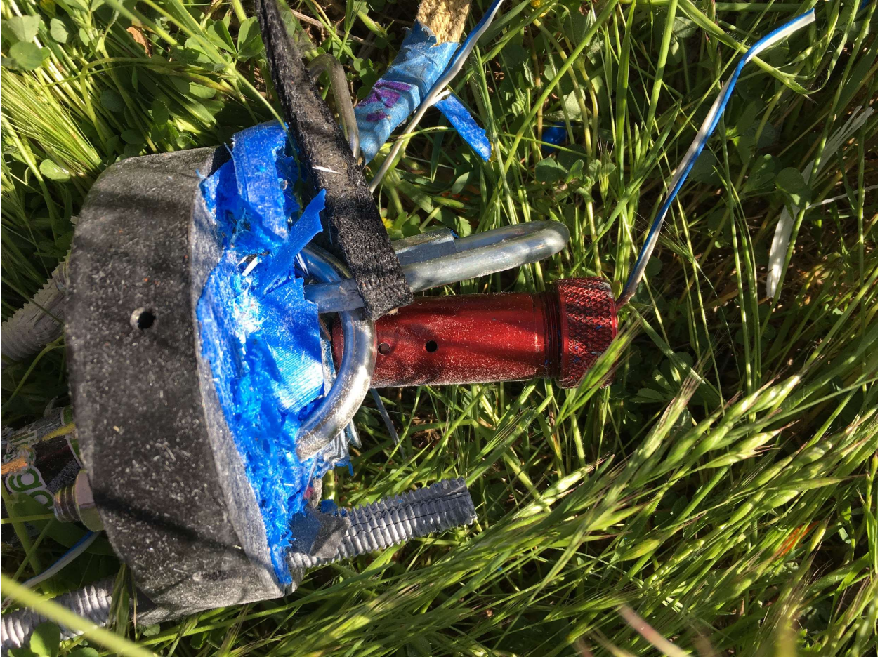
Drogue CO2 system still correctly set up post flight
