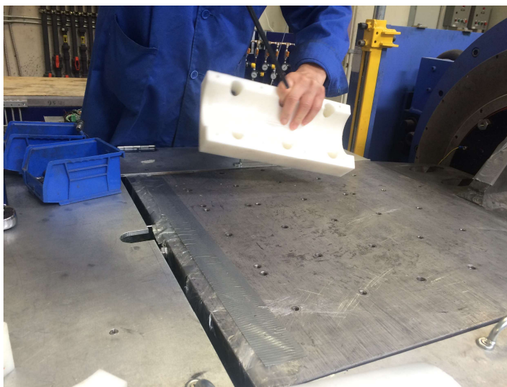
Fig. 1 - The shaker table, with the bottom half of the vibe jig pictured before being fixed
