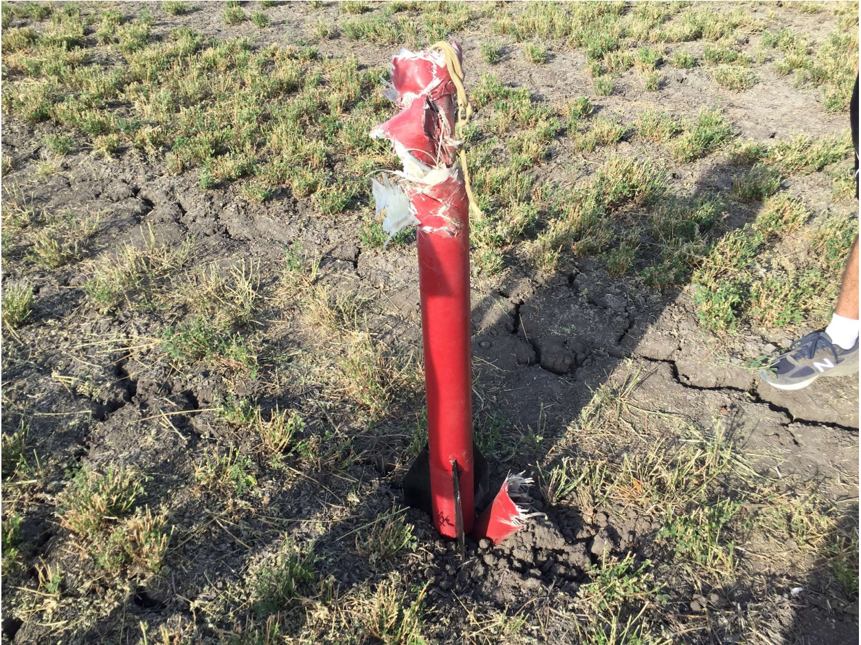
Aft frame with intersection shock cord ripped
