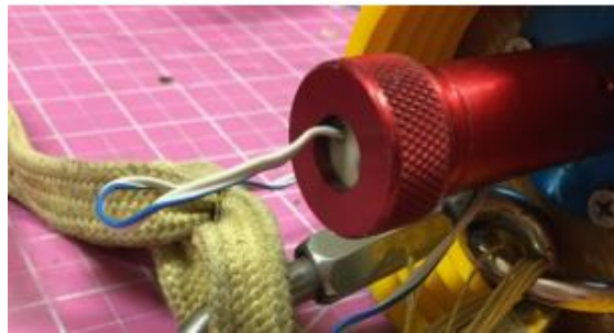
Figure 15. The CO 2 ejection mechanism used to pressurize and break the shear pins in the coupler that attaches the airframes.
