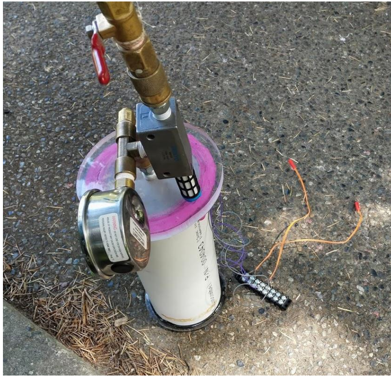
Fig 30. Set up for vacuum testing of Stratologger CF (inside container) with drogue and main parachute e-matches.
