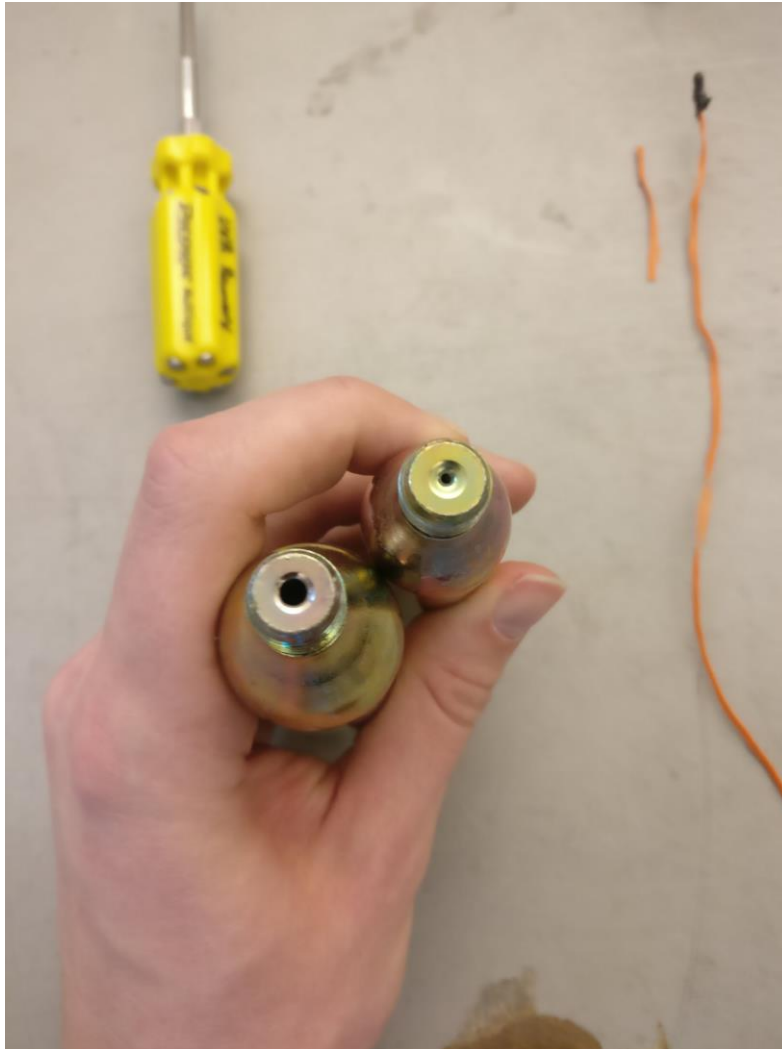
Figure 1: Optimal puncture (left) vs suboptimal puncture (right).
