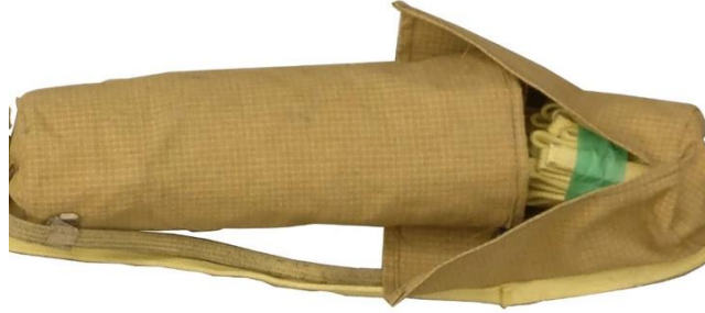
Fig 11. Custom 2-piece parachute bag enabling halves to split during main parachute deployment.
