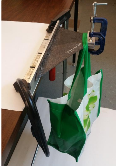
Fig 7. H1-5-21 in the static-bending strength test apparatus. Weights are suspended in a tote bag at the tip of the fin.
