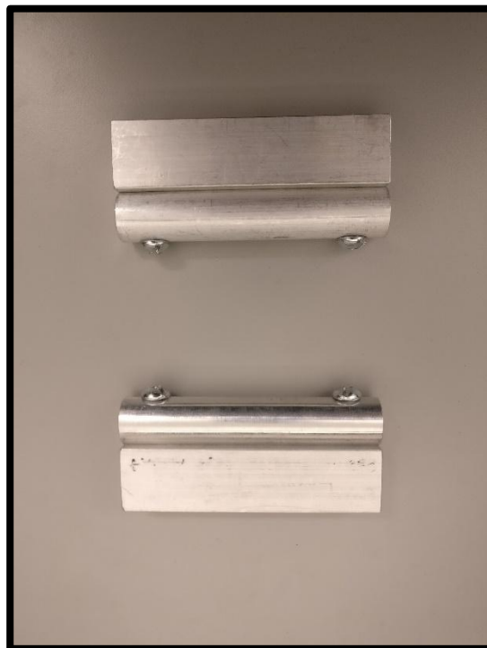
Figure 3: Custom test jig designed by Josiah Stefani. Fabric is squeezed between cylinder and block.
