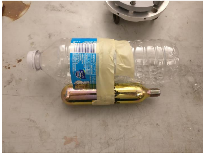
Figure 1: CO 2 cartridge attached to water bottle that acts as a floatation device
