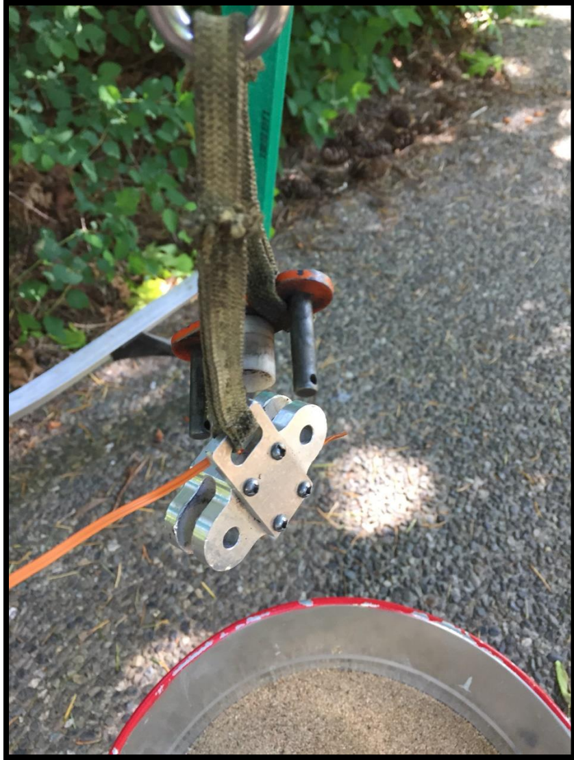
Figure 3: Clean separation of pyrelease, dropping the bucket.
