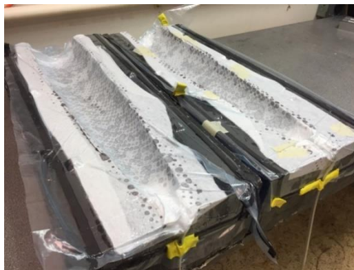
Fig 3. Test layup of nosecone halves, shown under vacuum.
