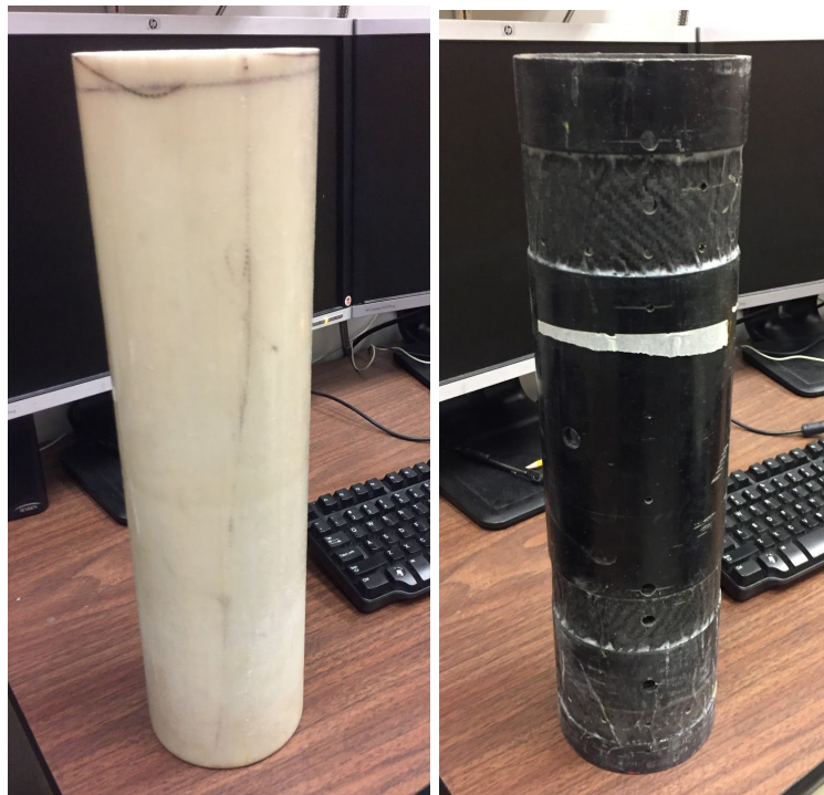
Figure 1: Foam-fibreglass coupler (left), ABS-fibreglass coupler (right)
