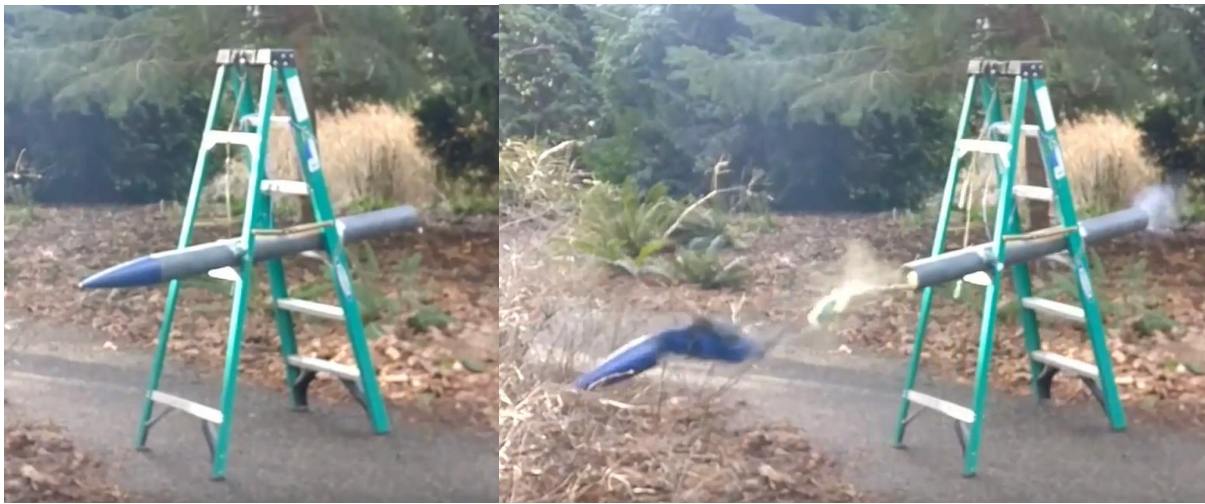
Figure 1: Nose cone deployment test jig, left. Nose cone successfully deployed, right
