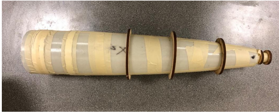
Fig 4. Picture of nose cone with laser cut rings.
