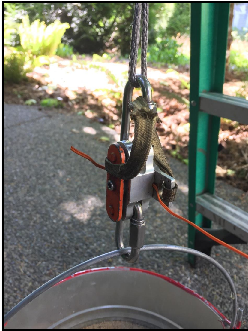
Figure 2: The pyrorelease holding the bucket against gravity.
