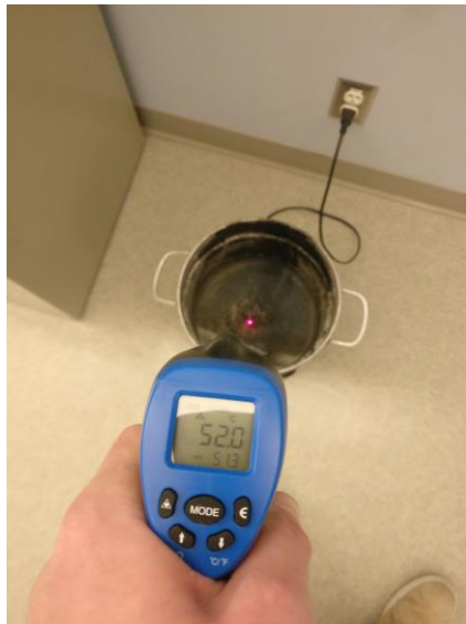
Figure 2: Heating up water and checking temperature with infrared thermometer
