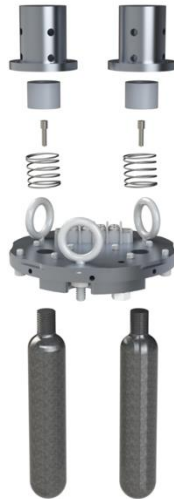
Fig 12. CO 2 ejection system. CO 2 cylinders threaded into puncture mechanism from below the bulkhead.
