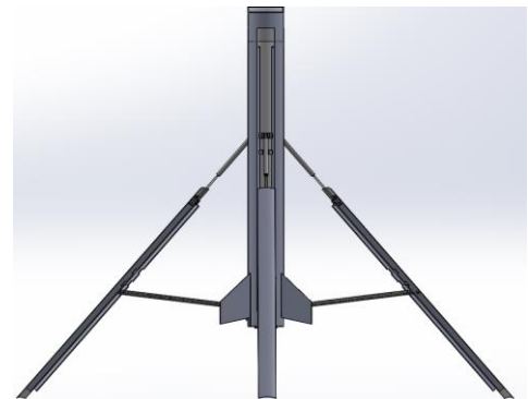
Figure 6. 3D model of landing leg subsystem.
