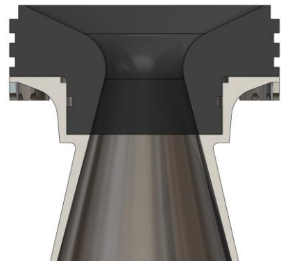
Figure 3: 3D Cross Section of Nozzle Assembly
