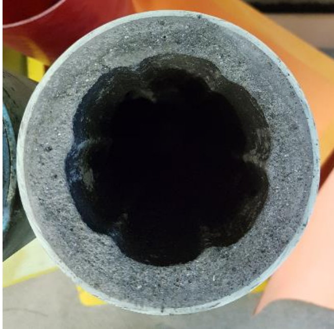
Figure 6. Kismet fuel grain after Static Fire 1. The unburned remaining HTPB can be seen insulating the walls of the liner, while the liner itself remained intact and undamaged following the burn.
