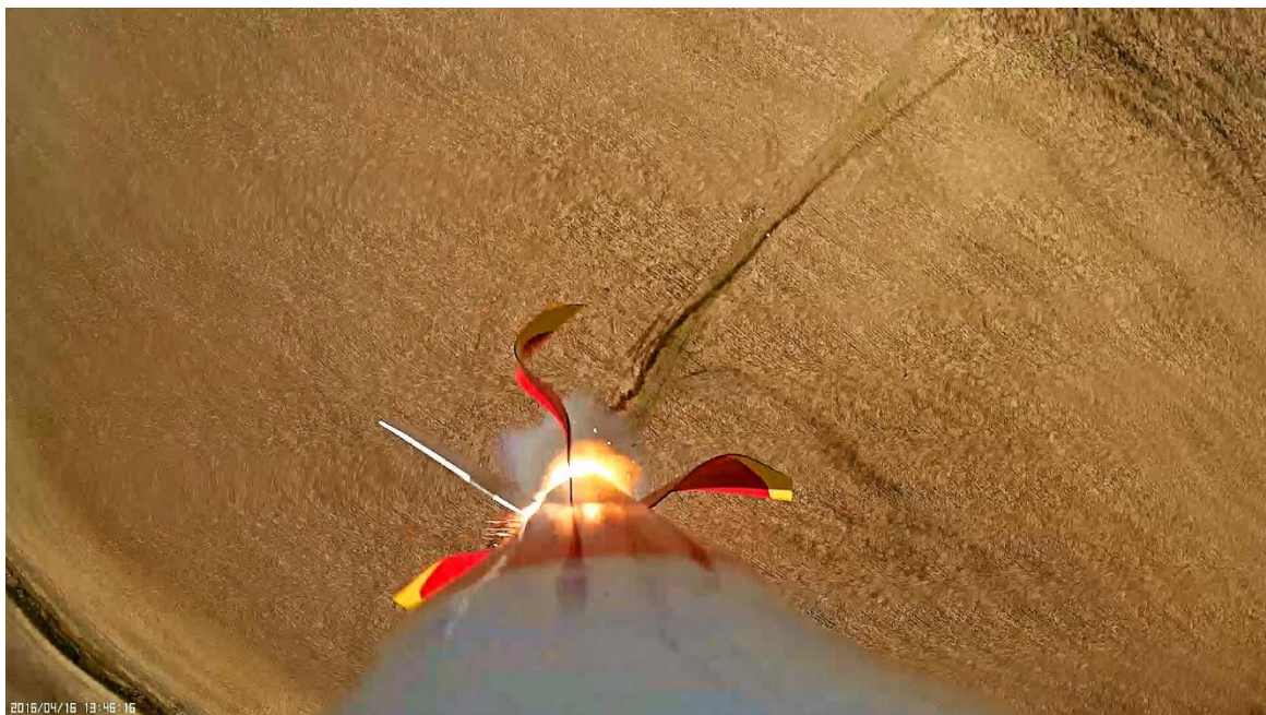
Figure 25. Fins flutter phenomena
