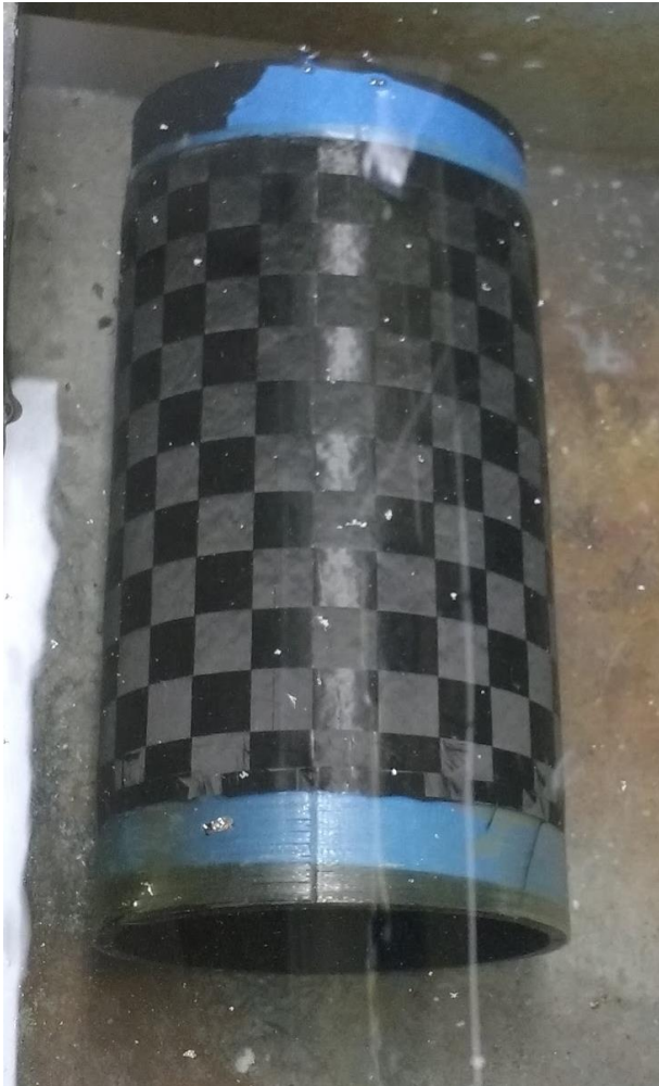
Figure 16. Carbon fiber test tube in water
