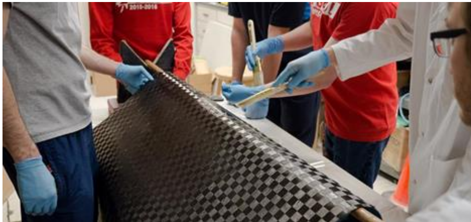
Figure 18. The team working on the wet layup process
