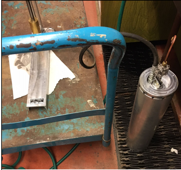
Figure 10. Combustion chamber assembly Hydro-test
