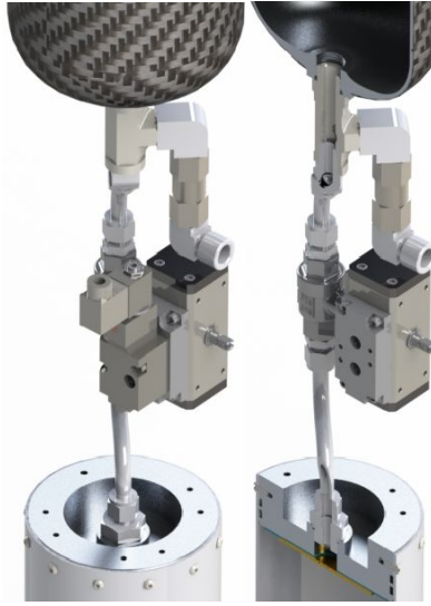
Figure 8. Assembled injector assembly with valves attached - full and cross-sectioned view
