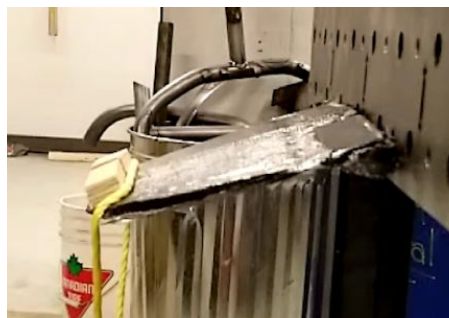
Figure 3: Fin Prototype just prior to failure
