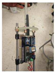
(b) Telemetry, diagnostics, and datalogging circuit
