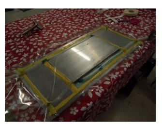
(a) Compressed fin preform under aluminum caul plate.
