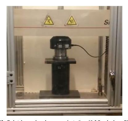
Figure 12 Body tube sample under compressive testing with failure load over 21,000 lbs.
