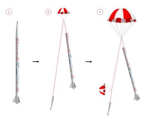
Figure 18 High-level recovery sequencing; including ascent, drogue descent, and main descent phases.
