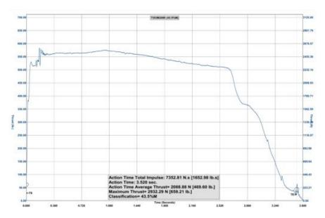
Figure 4 Thrust curve of COTS M2045 motor.
