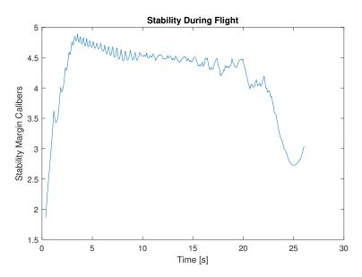
Figure 13 Stability evolution during flight.
