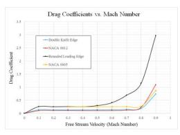
(b) Drag coefficients of various cross sections found using CFD.
