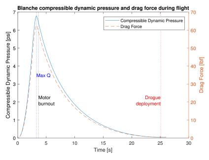
Figure 6 Blanche dynamic pressure and drag force during flight.
