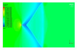
(a) Shockwave formation over a NACA0012 airfoil at M=0.9, a consideration against its use in the transonic range.
