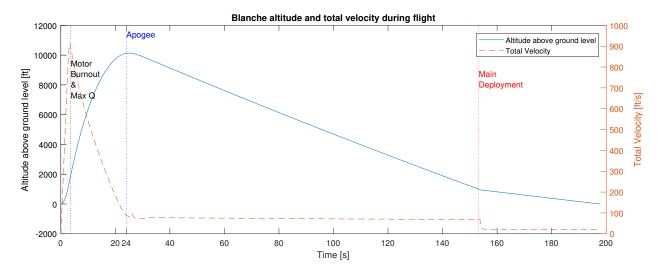
Figure 3 Blanche above ground altitude and total velocity during flight, with key flight events marked.
