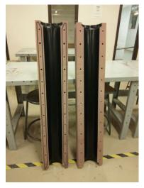
(a) Renshape molds after machining and coating.
