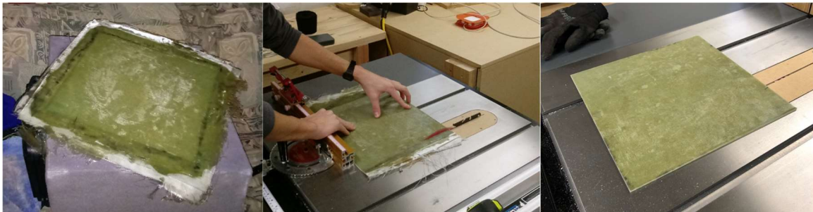
Figure 4. Stages of preparing a 12"x12" fiberglass sheet
