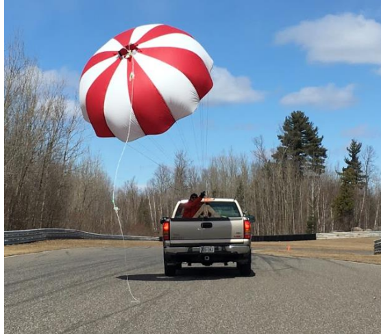
Figure 24. Successful parachute testing to measure drag and the drag coefficient.
