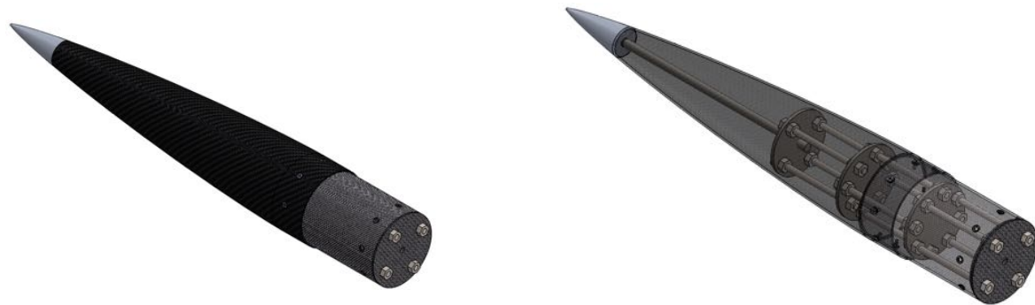
(a) von Karman CFRP nose cone design.
