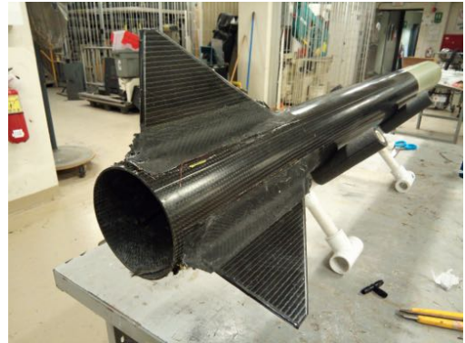
(c) Reinforced fins before finishing operations.
