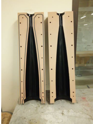
Figure 10 Renshape nose cone molds after finishing.
