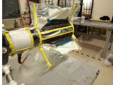
(b) Reinforcement under vacuum bag.
