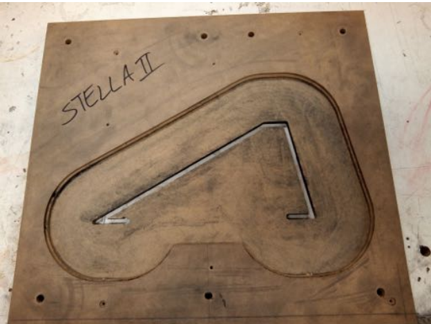
(b) Hand-held Router Cutting template for the fins.
