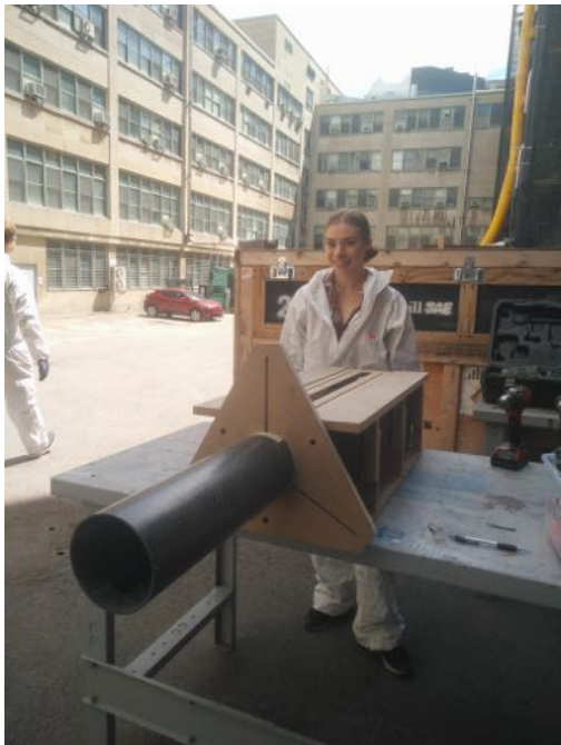
(a) Student made fin-slottting jig. Small human for scale.
