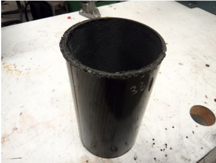
Figure 14 Failed body tube sample after compressive testing.
