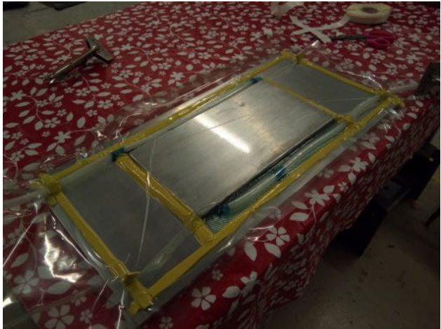
(a) Compressed fin preform under aluminum caul plate.
