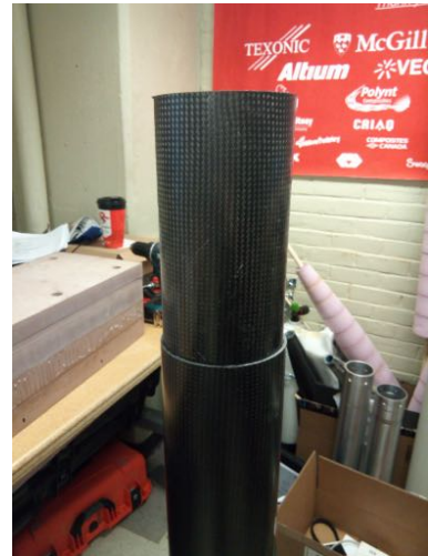
(c) Coupler fit with no sanding.
