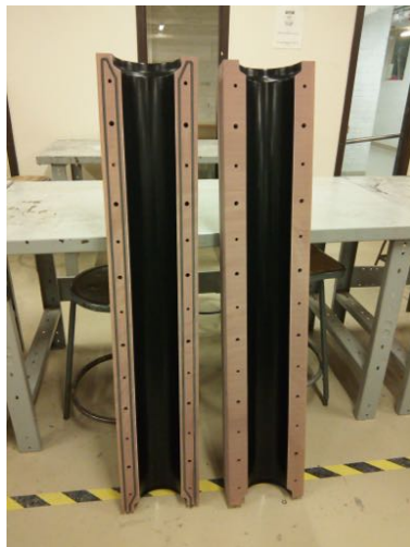
(a) Renshape molds after machining and coating.
