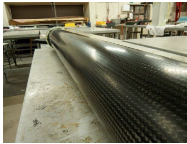
(b) Body tube after removal from the mold.
