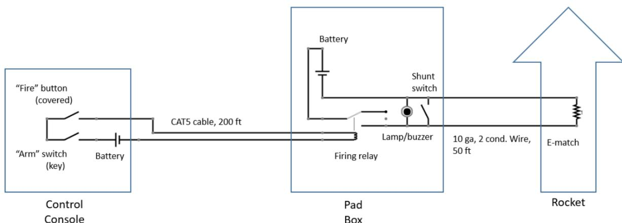
Figure 2: An improved high current fire control system.
