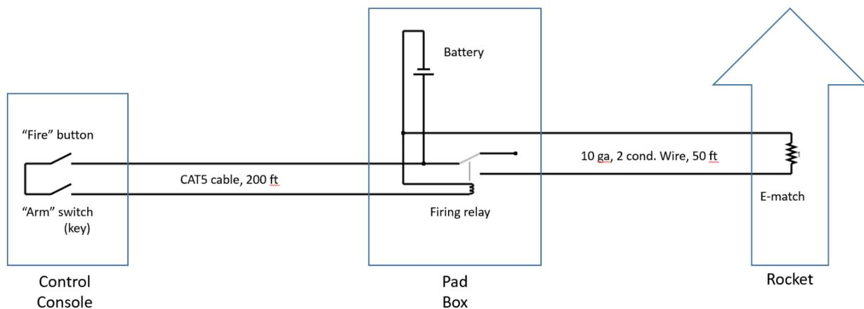
Figure 1: A simple high current fire control system.
